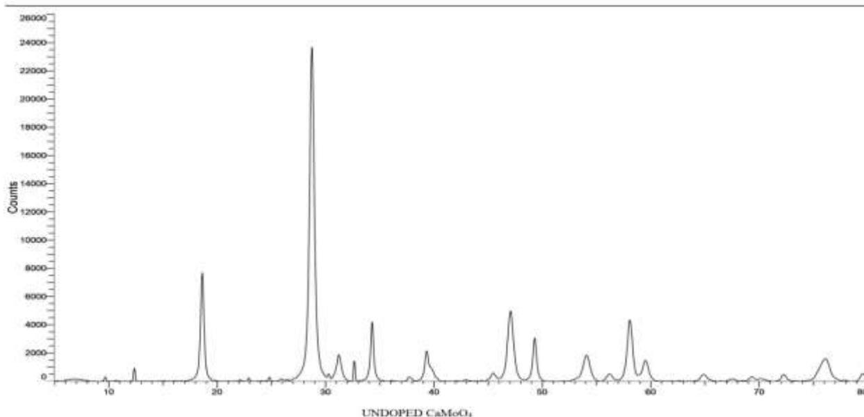
**Fig. 4: XRD of Undoped CaMoO<sub>4</sub>**
