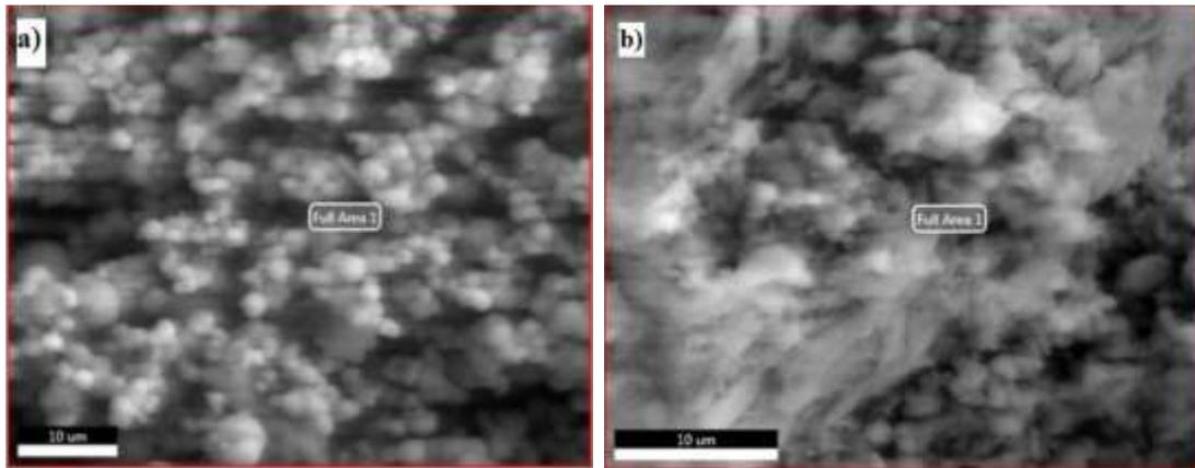
**Fig. 1: FE-SEM Images of (a) Undoped CaMoO<sub>4</sub> (b) 3% C-doped CaMoO<sub>4</sub>**
